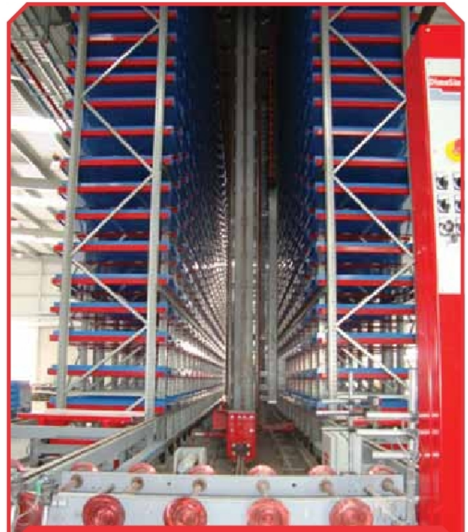
Example of execution of a warehouse for storing groups of complementary products in the loading units.
